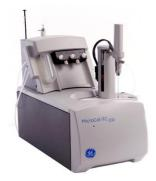
Isothermal Titration Calorimetry (ITC) is a popular technique for measuring bimolecular interactions. ITC determines all binding parameters (n, K,  $\Delta$ H and  $\Delta$ S) in a single experiment – information, simultaneously that in not possible with any other method. We have Microcal iTC200 for various applications which includes
