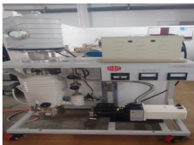
Pumping system for vacuum seal attached with Thermal Evaporation for metallic thin film
