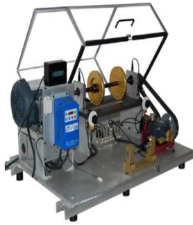
7. Machinery Fault Simulator (Model: MFS 2010 PK-7 from Spectraquest Inc. USA): Procured and installed
