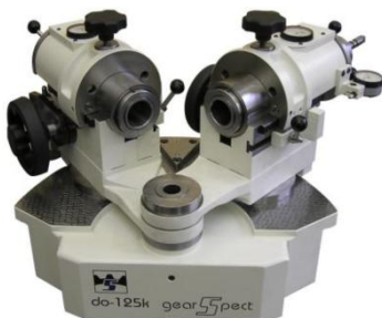
3. Computerized Double Flank Gear Roll Tester (Model: DO 125 K PC): Procured and installed
