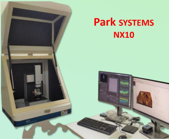
Electrostatic Force Microscopy (EFM), Scanning Kelvin Probe Microscopy (SKPM), and Piezoelectric Force Microscopy (PFM) are important electrical modes of Atomic Force Microscopy that extend surface characterization beyond topography to probe functional properties at the nanoscale.
