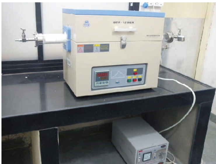
Single zone split-tube furnace (1200°C)
