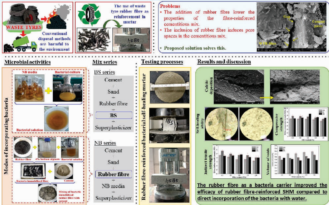
Micro and macro-structural properties of waste tyre Rubber Fibre-Reinforced Bacterial self-healing mortar
